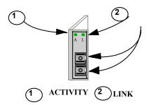
and with no cable connected. The FX port emits light outside of the visible spectrum and will always look dark to the human eye.
